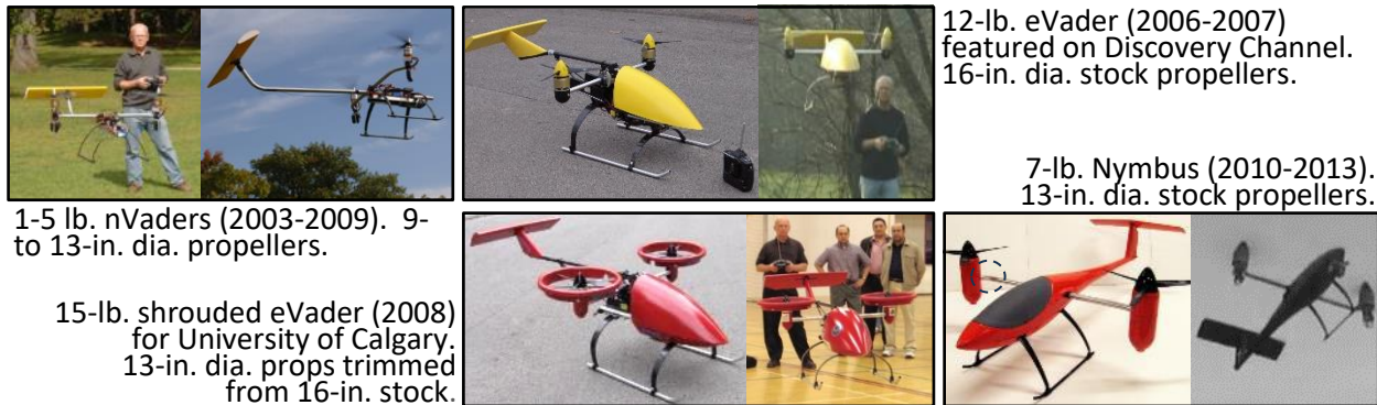
Fig. 14. Several of the oblique active tilting (OAT) bicopters designed and built by author.
